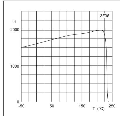
Fig. 2 Initial permeability as a function of temperature
