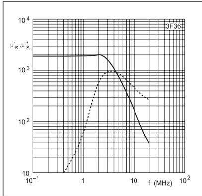
Fig. 1 Complex permeability as a function of frequency
