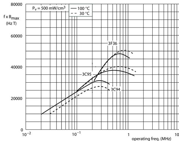
The performance factor ( $f \times B_{max}$ ) is a measure of the throughput power that a ferrite core can handle at a certain loss level.
