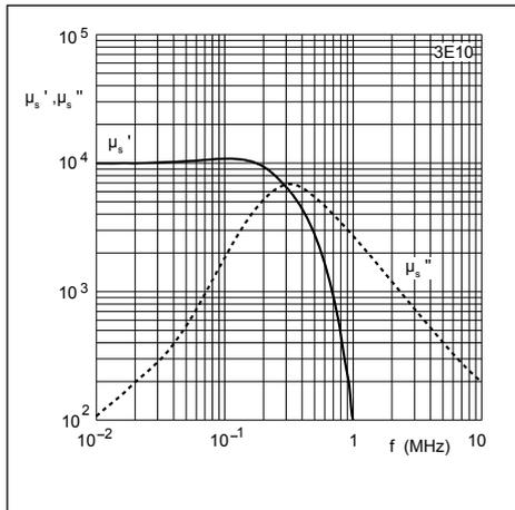
Fig. 1 Complex permeability as a function of frequency
