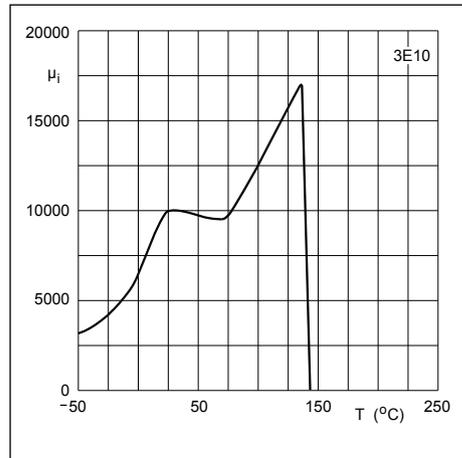
Fig. 2 Initial permeability as a function of temperature
