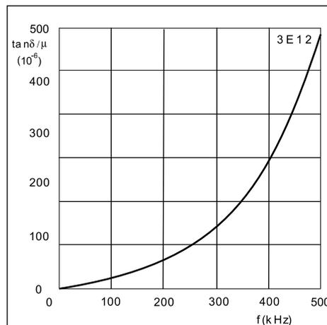
Fig. 6 Loss factor in function of frequency
